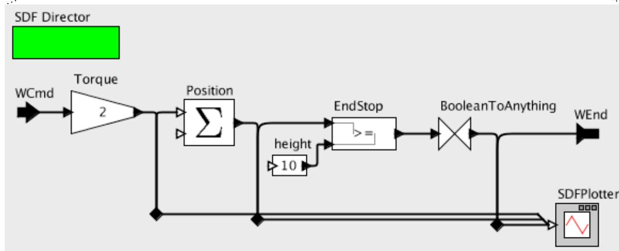
*Model of the window in “open loop”: up mode with up endstop detection*
